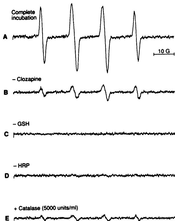
Fig. 6. ESR spectrum of the DMPO/glutathione thiyl radical adduct produced in a system of clozapine and HRP. A, Incubation containing 100 \mu M clozapine, 10 mM glutathione, 100 mM DMPO, 25 \mu g/ml HRP, and 0.5 mM DTPA, in 0.05 M phosphate buffer, pH 7.4. B, Same as in A, but without addition of clozapine. C, Same as in A, but without glutathione. D, Same as in A, but without HRP. E, Same as in A, but with the addition of 5000 units/ml catalase. The instrumental conditions were as follows: 20 mW microwave power, 0.6 G modulation amplitude, 0.160 sec time constant, and 40 G/min scan rate.
